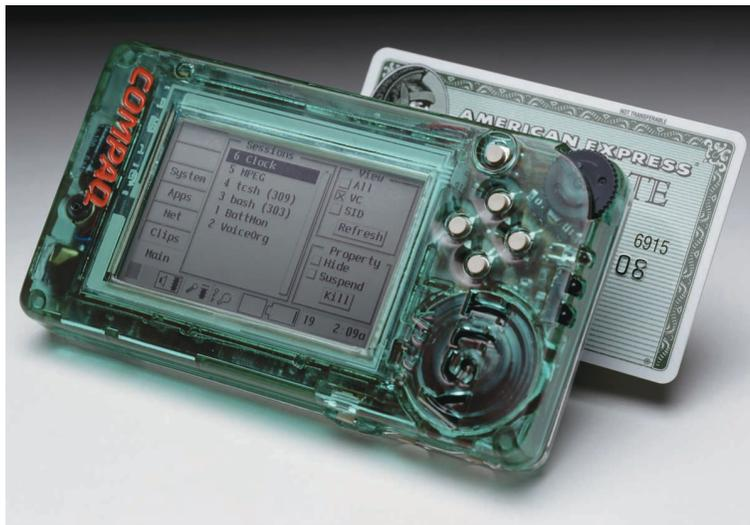
**Figure 4.** A session manager running on Itsy v2. Several applications are simultaneously running in the background, including an MPEG player, a battery monitor, and a voice organizer.
